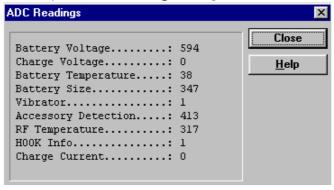
ADC Readings dialog has static text field where measurements are updated every second.
